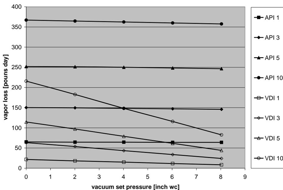
**Fig. 2 Vapor losses in function of vapor vacuum for various tank volumes**
