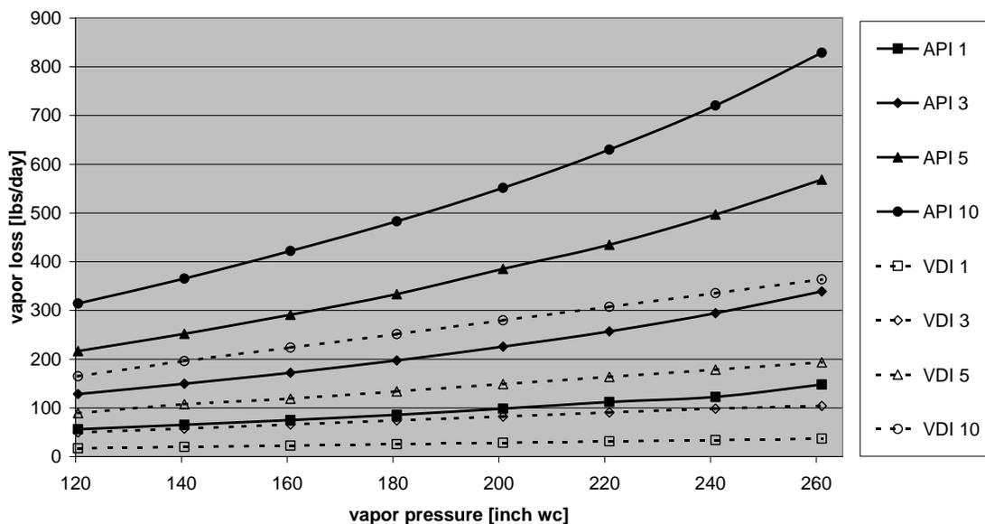
**Fig. 1 Vapor losses in function of vapor pressure for various tank volumes**
