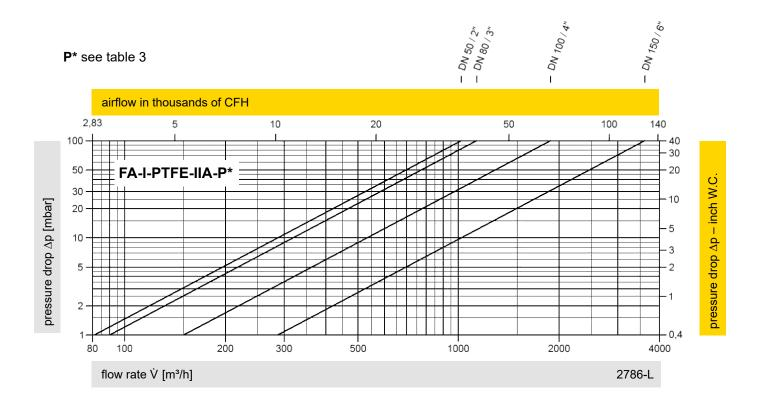
The flow capacity charts have been determined with a calibrated and TÜV certified flow capacity test rig. Volume flow  $\dot{V}$  in (m³/h) and CFH refer to the standard reference conditions of air in ISO 6358 (20°C, 1bar). For conversion to other densities and temperatures, refer to Sec. 1: "Technical Fundamentals."
